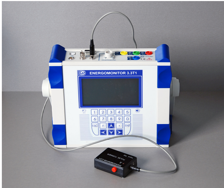
Fig. C.11. Pulse Former connected for testing meters of induction (disk) type (a pulse is generated on each press of the button)
