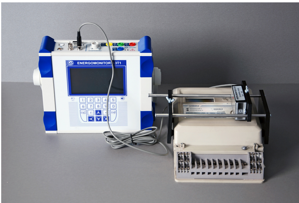
Fig. C.10. Attaching a meter with optical pulse output via SH-E scanning head
