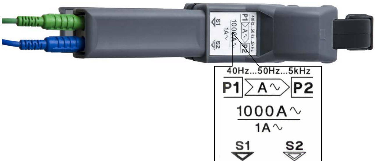
Fig. B.4. Stenciled marks “source → load” on a 1000A Current Clamp
