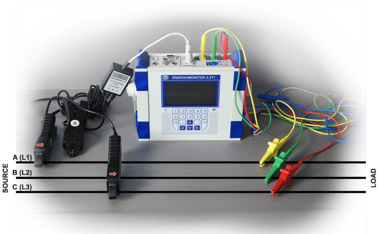
Fig. C.6. Three-phase 3-wire connection via a Current Clamp kit
