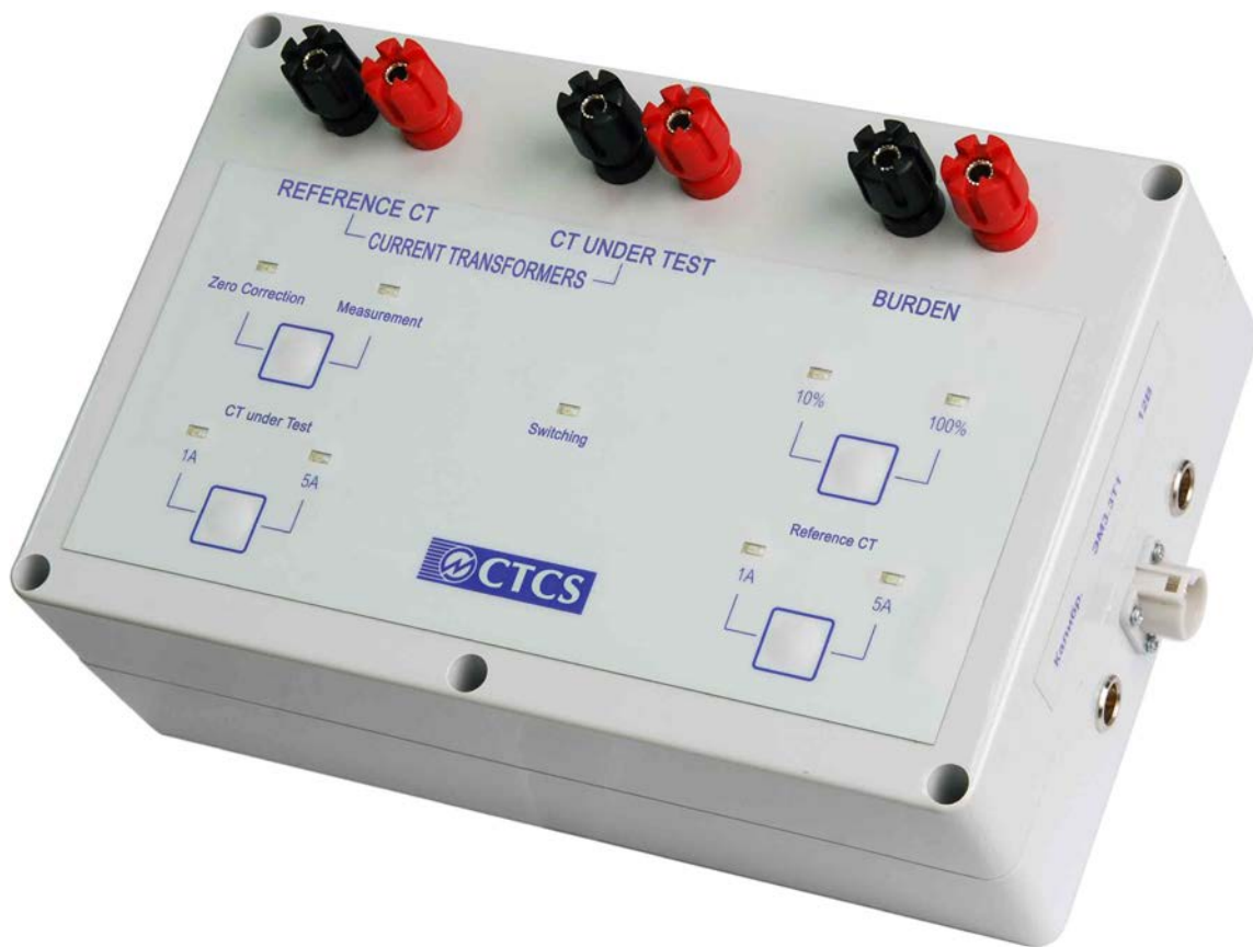
Fig. 4.46. CTCS (5 A): Terminals to be connected to external devices; controls and indicators
