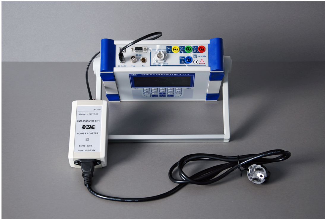
Fig. C.1. Connecting the EM-3.3T1 to mains via power adapter
