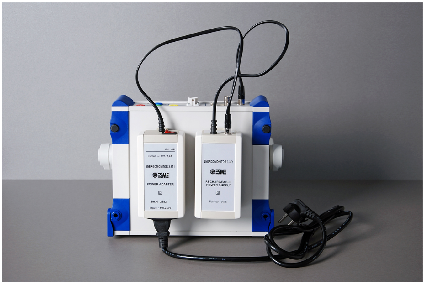
Рис. C.2. Connecting the EM-3.3T1 to mains via Power adapter and the Rechargeable power supply
