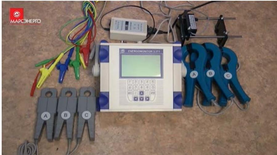
Fig. 2 Reference Standard Energomonitor 3.3T1 with its meter test kit
