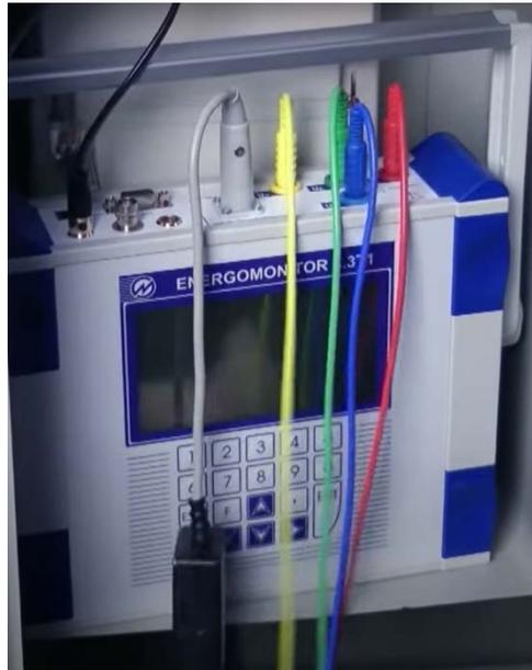
Fig. 4 Connecting output of current clamps to the EM
