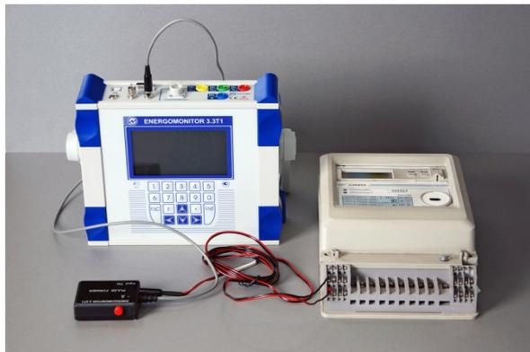
Fig. 10 Connecting tested meter to the EM via PF
