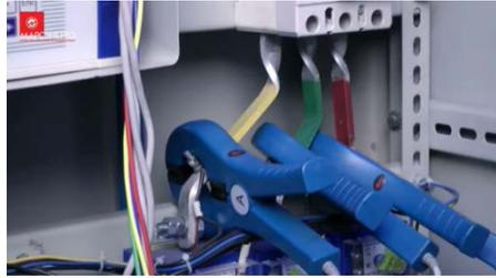
Fig. 6 Current clamps clamped around the primary wires of the CTs
