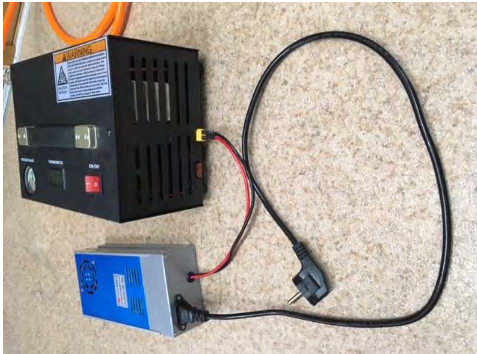
Fig. 4 Powering the compressor from the 220V mains supply
