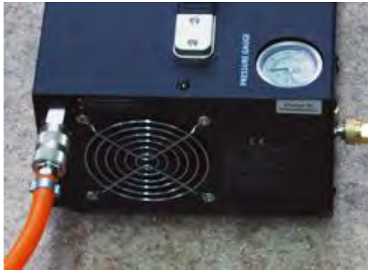
Fig. 9 Connecting the gas pipe to the Compressor
