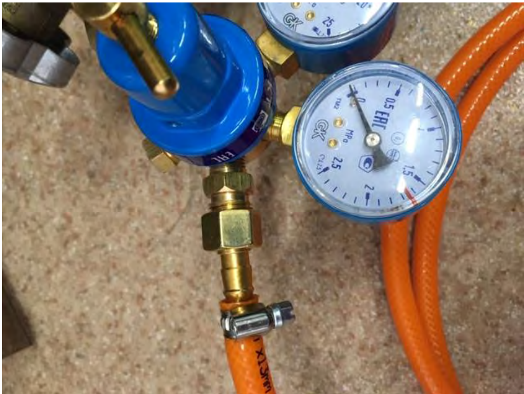
Fig. 2 Connecting the gas pipe to the Pressure Reduction unit
