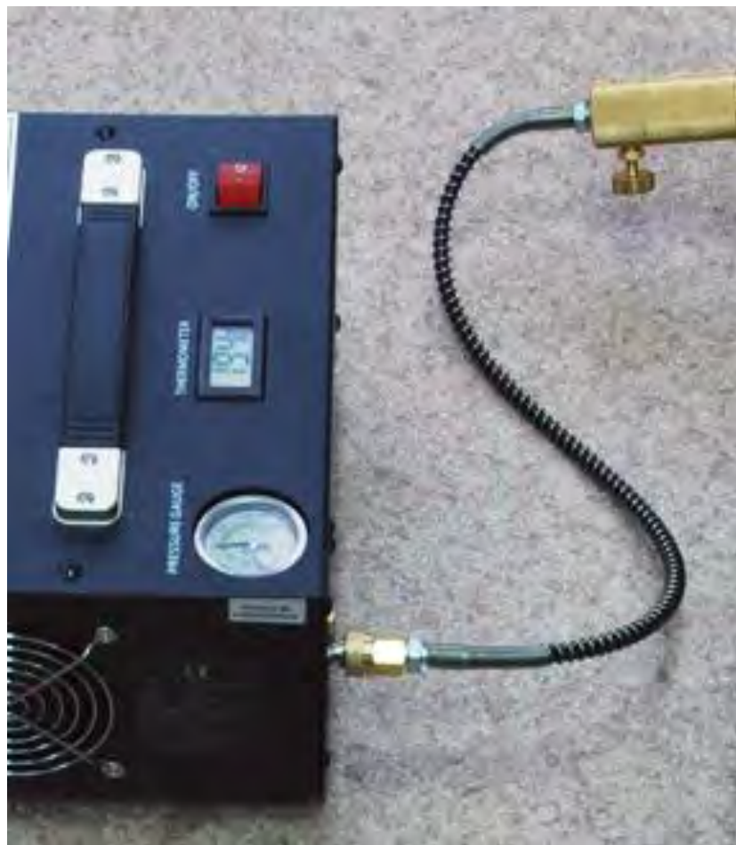
Fig. 6 Connecting the outlet pipe of the Compressor
