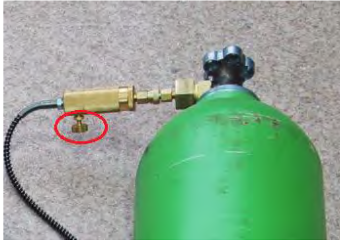
Fig. 11 Protective valve on the filter of the Compressor
