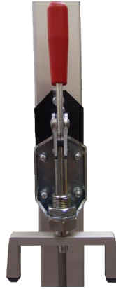
Fig. 4 Holder for fixing the meter in vertical plane
