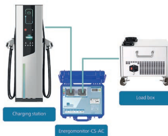
Fig. Charging station tested at a resistive load
