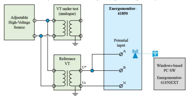
Connection scheme for zero correction of analogue current transformers:
